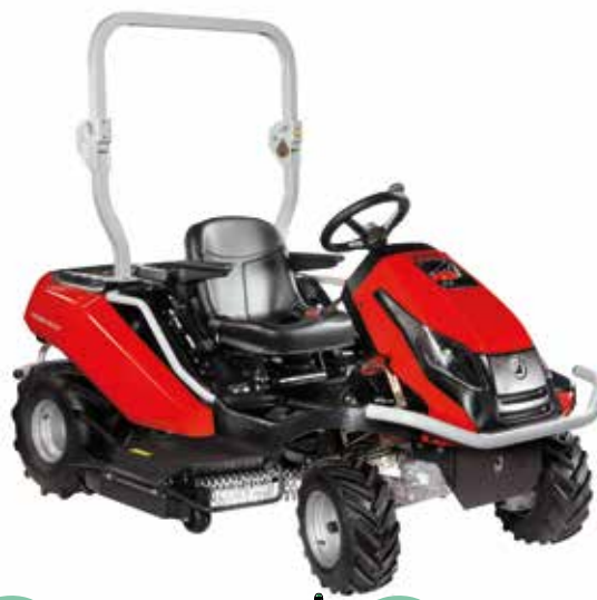
Equipped as standard with roll bar, front and rear bumpers, side guards and seat belt to ensure maximum safety, even when tackling the most complex situations ( TONKAWA ).
