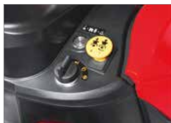
The electromagnetic clutch is engaged quickly and quietly by way of a handy dash-mounted button.
