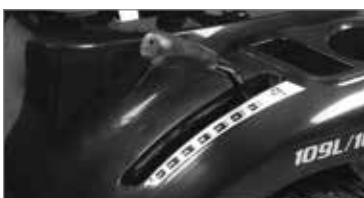
Practical cutting height adjustment with a conveniently positioned lever, with a graduated scale to show the cutting height at a glance.
