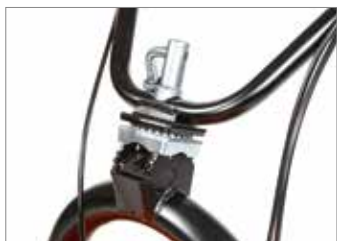
Handlebar with vertical and horizontal adjustment using the handlebar-mounted lever.
