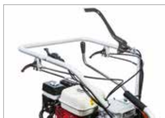
Steering with independently controlled release and brakes.
