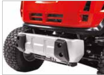
Generously sized front bumper in steel for high strength and resistance in the case of accidental impact.
